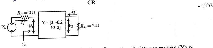
For the two-port network shown in the above figure, the admittance matrix (Y) is shown. Find-
